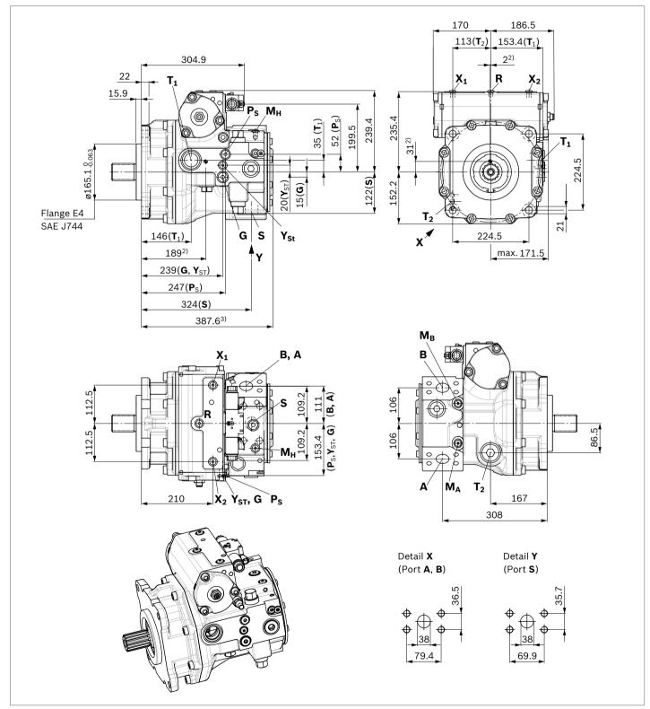
$_{\rm 1)}$  For SAE working ports  ${\bf A}$  and  ${\bf B},$   $45^{\circ}$  right (viewed on drive shaft), the complete case and thus the dimensions are mirrored.
